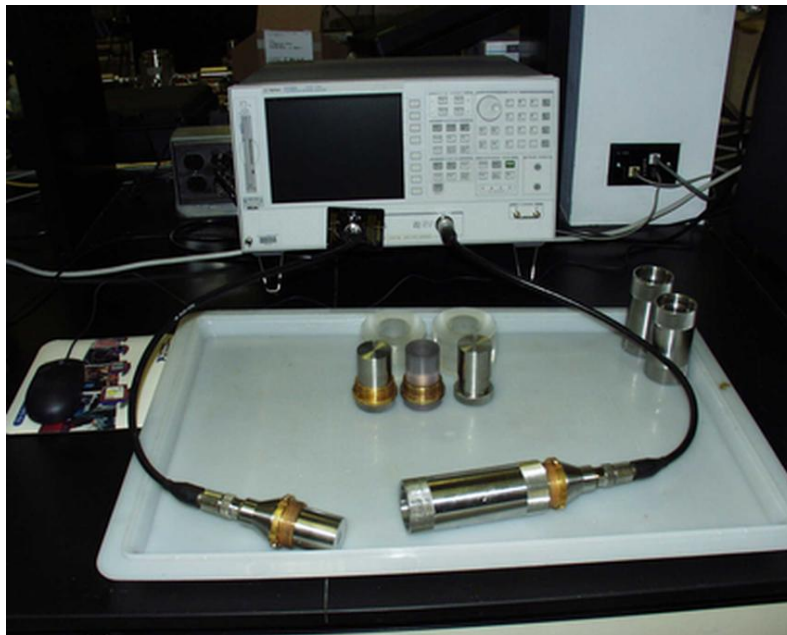
Fig. 1. Cylindrical dielectric cell connected to a network analyzer.
