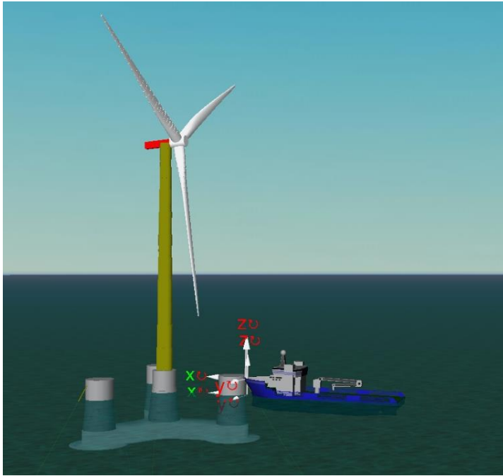
Figure 11. Global ship-FOWT collision analysis setup
